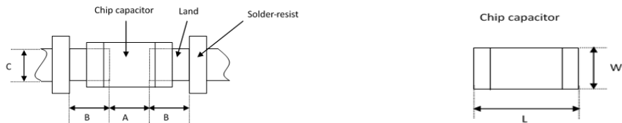
Recommended land dimensions for reflow-soldering
